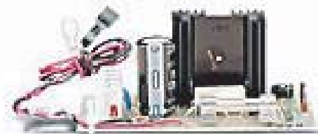
12V, 1A Power Supply (ADEMCO AD12612 or equivalent)
